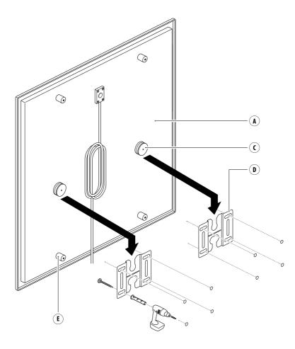
8. Turn the four **spacers**(E) to lock the **infrared heater** in place.
